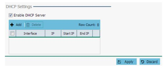
20. Select Enable DHCP Server to ensure the Access Point can provision IP addresses to requesting clients over the specified interface.
