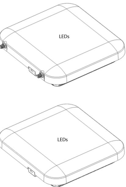
The LEDs provide a status display indicating error conditions, transmission, and network activity for the 5 GHz 802.11ac (amber) radio and the 2.4 GHz 802.11n (green) radio.
