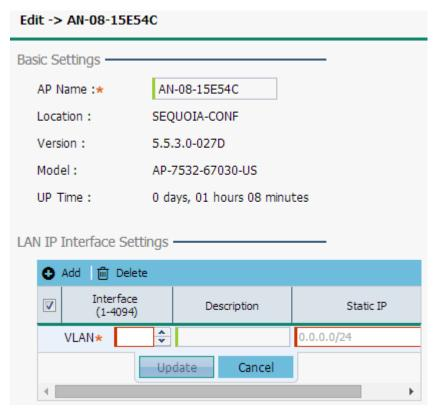
Refer to the **LAN IP Interface Settings** field, and add a VLAN and Static IP as required for enabling DHCP (within the *Configuration* > *Services* screen) for client IP address requests and ensuring routable traffic.
